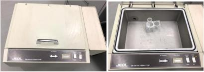
3.11 Close the lid. And check that the vent valve is pointed horizontal as shown.
