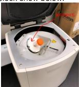
3.3 Insert a clean vial (supplied by the NRF) and place on top of the digital scale and insert new mixing vial, remove the orange top.
