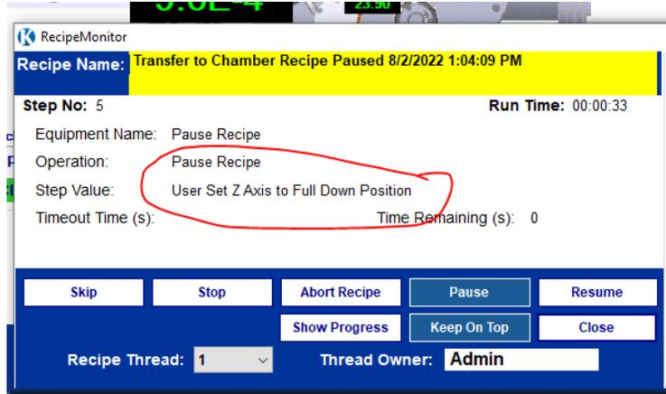
4.13 When “Pause – User Confirm Z-Shift Position” appears in the “Step” field, verify that the platen is all the way down. See red arrow in pic below. Normally it is already in this position from the last user.
