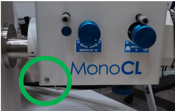
Green Light ....The mirror is fully retracted
